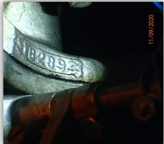
7a. 100M Front Intake Manifold 1B2893
