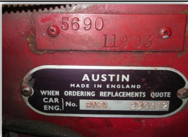
4/5. Batch/Body and Car/Engine Number Plates With Correct Phillips Screws
