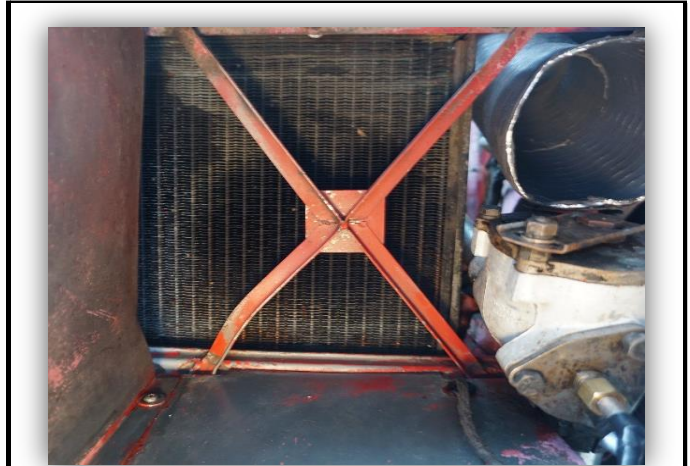
11. 100M Bent Brace For Cam Installation
