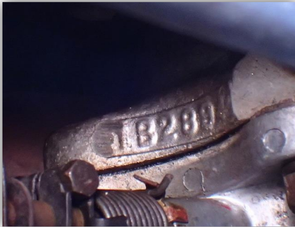
7b. 100M Rear Intake Manifold 1B2894
